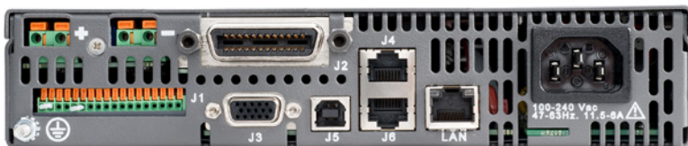
Rear panel of the 60V and higher voltage versions showing the terminal block output connectors and all analog and digital interface connectors.
